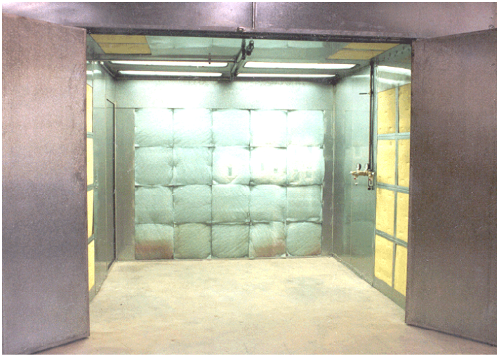
Typical Dry Filter, Cross Draft Type Booths
